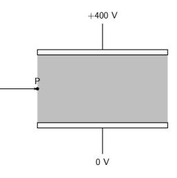
A potential difference of 400 V is applied across the places which are separated by 8 mm. The electric field intensity in the shaded region between the metal plates is uniform. Outside this region, it is zero.
