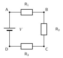
The first principle to understand about series circuits is that the amount of current is the same through any component in the circuit. This is because there is only one path for electrons to flow in a series circuit. From the way that the battery is connected, we can tell which direction the current will flow. We know that current flows from positive to negative, by convention. Current in this circuit will flow in a clockwise direction, from point A to B to C to D and back to A.
