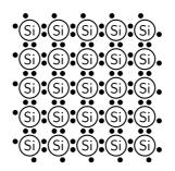
Figure 20.1: Arrangement of atoms in a Si crystal.
