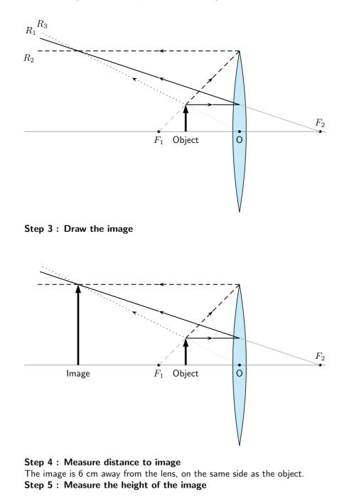
The image is 3 cm high. **Step 6 : Is image real or virtual?** Since the image is on the same side of the lens as the object, the image is virtual.
