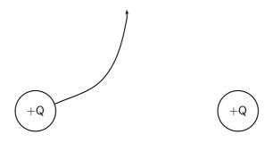
We know that a charge the same distance below the middle will experience a force along a reflected line, because the problem is symmetric (i.e. if we flipped vertically it would look the same). This is also true in the horizontal direction. So we use this fact to easily draw in the next four lines.
