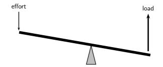
Figure 12.21: A lever is used to put in a small effort to get out a large load.
