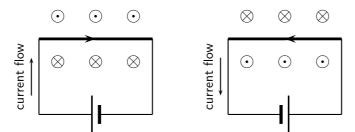
Figure 18.2: Magnetic fields around a conductor looking down on the conductor. (a) Current flows clockwise. (b) current flows counter clockwise.
