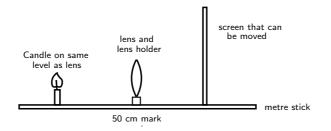
Figure 13.6: Experimental setup for investigation.
