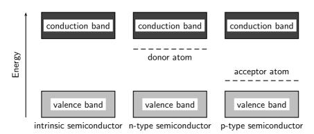
The energy level of the donor atom is close to the conduction band and it is relatively easy for electrons to enter the conduction band. The energy level of the acceptor atom is close to the valence band and it is relatively easy for electrons to leave the valence band and enter the vacancies.
