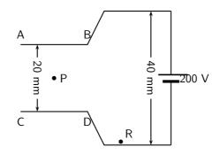
When a charged particle Q is placed at point R, it experiences a force of magnitude F. Q is now moved to point P, halfway between plates AB and CD. Q now experiences a force of magnitude .
