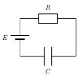
Figure 17.1: A capacitor (C) connected in series with a resistor (R) and an energy source (E).
