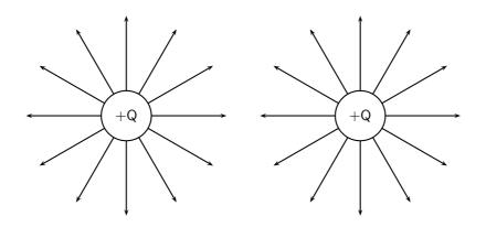
The field directly between the charges cancels out in the middle. The force has equal magnitude and opposite direction. Interesting things happen when we look at test charges that are not on a line directly between the two.
