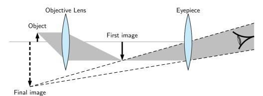
Figure 13.21: Compound microscope
