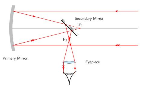
Figure 13.20: Lenses and mirrors in a reflecting telescope.
