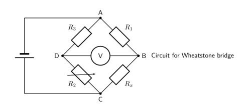
In the circuit of the Wheatstone bridge,  $R_x$  is the unknown resistance.  $R_1$ ,  $R_2$  and  $R_3$  are resistors of known resistance and the resistance of  $R_2$  is adjustable. If the ratio of  $R_2:R_1$  is equal to the ratio of  $R_x:R_3$ , then the voltage between the two midpoints will be zero and no current will flow between the midpoints. In order to determine the unknown resistance,  $R_2$  is varied until this condition is reached. That is when the voltmeter reads 0 V.
