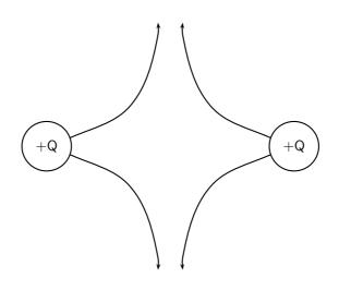
Working through a number of possible starting points for the test charge we can show the electric field map to be:
