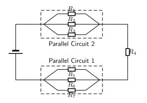
Figure 19.1: An example of a series-parallel network. The dashed boxes indicate parallel sections of the circuit.
