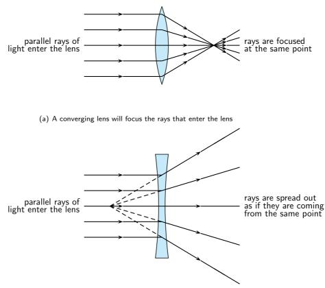
(b) A diverging lens will spread out the rays that enter the lens
