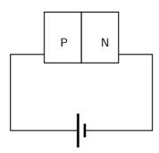
The electric field from the external potential different can easily overcome the small internal field (in the so-called depletion region, created by the initial drifting of charges): usually anything bigger than 0.6V would be enough. The external field then attracts more e- to flow from n-region to p-region and more holes from p-region to n-region and you have a forward biased situation. the diode is forward biased and so current will flow.
