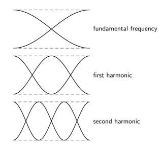
Figure 16.2: Harmonics in a pipe open at both ends.
