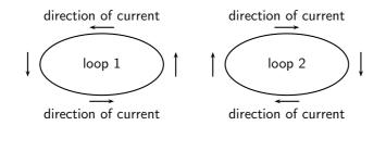
If you make a loop of current carrying conductor, then the direction of the magnetic field is obtained by applying the Right Hand Rule to different points in the loop.
