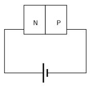
In this case the external field pushes e- back to the n-region while more holes into the p-region, as a result you get no current flow. Only the small number of thermally released minority carriers (holes in the n-type region and e- in the p-type region) will be able to cross the junction and form a very small current, but for all practical purposes, this can be ignored.
