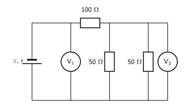
The resistances of voltmeters  $\mathsf{V}_1$  and  $\mathsf{V}_2$  are so high that they do not affect the current in the circuit.
