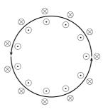
The directions of the magnetic field around a loop of current carrying conductor with the current flowing in a counter-clockwise direction is shown.
