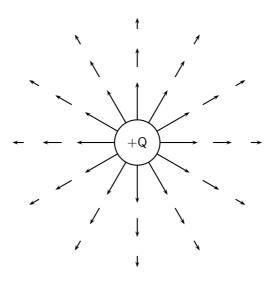
We can see that at every point the positive test charge, q, would experience a force pushing it away from the charge, Q. This is because both charges are positive and so they repel. Also notice that at points further away the vectors are shorter. That is because the force is smaller if you are further away.
