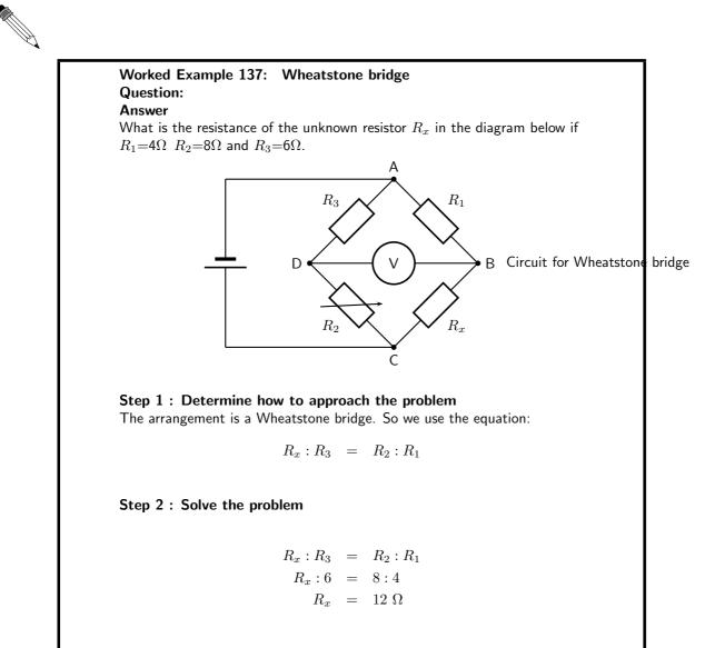
**Step 3 : Write the final answer** The resistance of the unknown resistor is  $12 \Omega$ .
