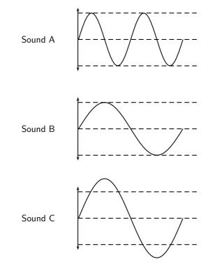
Figure 15.1: Pitch and loudness of sound. Sound B has a *lower* pitch (lower frequency) than Sound A and is *softer* (smaller amplitude) than Sound C.
