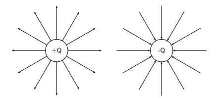
Notice that a test charge starting off directly between the two would be pushed away from the positive charge and pulled towards the negative charge in a straight line. The path it would follow would be a straight line between the charges.
