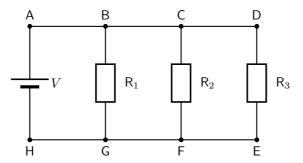
The first principle to understand about parallel circuits is that the voltage is equal across all components in the circuit. This is because there are only two sets of electrically common points in a parallel circuit, and voltage measured between sets of common points must always be the same at any given time. So, for the circuit shown, the following is true:
