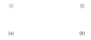
Figure 18.1: Magnetic field around a conductor when you look at the conductor from one end. (a) Current flows out of the page and the magnetic field is counter clockwise. (b) Current flows into the page and the magnetic field is clockwise.
