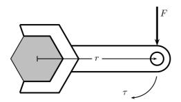
Figure 12.19: The force exerted on a spanner helps to loosen the bolt.
