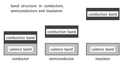
Electrons follow the Pauli exclusion principle, meaning that two electrons cannot occupy the same state. Thus electrons in a solid fill up the energy bands up to a certain level (this is called the Fermi energy). Bands which are completely full of electrons cannot conduct electricity, because there is no state of nearby energy to which the electrons can jump. Materials in which all bands are full are insulators.
