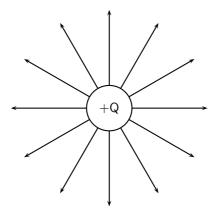
Notice that as you move further away from the charge the field lines become more spread out. In field map diagrams, the closer together field lines are, the stronger the field. Therefore, the electric field is stronger closer to the charge (the electric field lines are closer together) and weaker further from the charge (the electric field lines are further apart).
