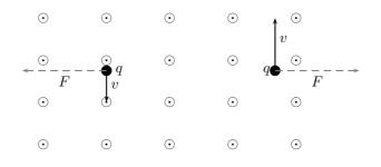
Worked Example 129: Charged particle moving in a magnetic field Question: An electron travels at  $150 \text{m.s}^{-1}$  at right angles to a magnetic field of 80 000 T. What force is exerted on the electron? Answer Step 1 : Determine what is required We are required to determine the force on a moving charge in a magnetic field Step 2 : Determine how to approach the problem We can use the formula: F = qvB
