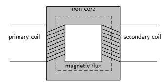
When an alternating voltage is applied to the primary coil it creates an alternating current in that coil, which induces an alternating magnetic field in the iron core. The changing magnetic flux through the secondary coil induces an emf, which creates a current in this secondary coil.
