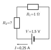
Step 7 : Determine how to approach the problem. We can use Ohm's Law to find the total resistance R in the circuit, and then calculate the unknown resistance using:
