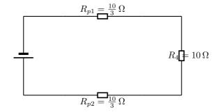
This has now being simplified to a simple series circuit and the equivalent resistance is:
