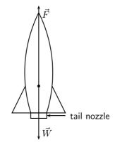
The rocket accelerates because the magnitude of the upward force, F is greater than the magnitude of the rocket's weight, W. Which of the following statements **best** describes how force F arises?
