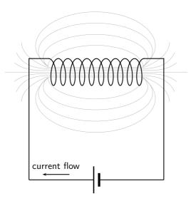
Figure 18.4: Magnetic field around a solenoid.
