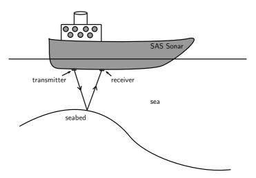
Ships on the ocean make use of the reflecting properties of sound waves to determine the depth of the ocean. A sound wave is transmitted and bounces off the seabed. Because the speed of sound is known and the time lapse between sending and receiving the sound can be measured, the distance from the ship to the bottom of the ocean can be determined, This is called sonar, which stands from **So**und **N**avigation **And R**anging.
